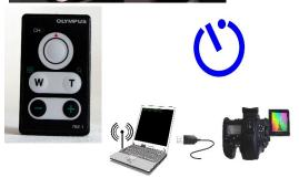
Blurred images are mostly caused by releasing the shutter manually. This leads to **vibrations**, which are picked up as motion blurs in the images. To avoid motion blurs, we recommend that you use a **remote control** release. Otherwise it is also possible to use the digital camera's self-timer function.
