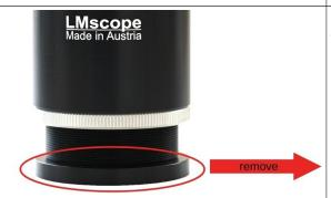
To expand the available range of uses, a 5 mm C-mount extender is included with this microscope adapter. If you are working with instruments that do not conform to the C-mount standard, you can remove the extender.
