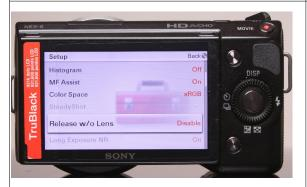
Some cameras by default require a lens to be attached in order to release the shutter. If this is the case with your camera, select the "release without lens" option in the camera menu (wording varies from manufacturer to manufacturer).
